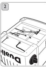
Loosen locking nuts on Unscr retaining plate using a 6.5mm wires. spanner and slide back.
