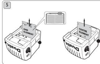
Remove element. To re-assemble, reverse procedure ensuring wires and parts are correctly positioned. Ensure new element is marked the same as the one removed and is seated correctly in the channels either side. PAT test before use.
