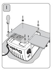
Unplug and place toaster on a soft cloth. Remove crumb tray and unscrew feet to remove the base plate.
