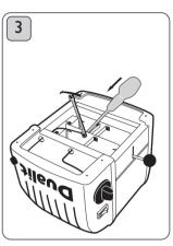
Unscrew brass links and wires.
